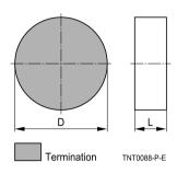
$D = 3.5 \pm 0.3 \text{ mm}$  $L = 1.3 \pm 0.4 \text{ mm}$
